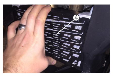
Peel the backer off of the adhesive strips, carefully place the guard over the oil cooler like you did in step 3. Press firmly on the top and bottom flanges to ensure good contact of the adhesive. Put the belly pan back on.
