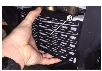
Before you peel the backing off ot he high temp adhesive do a test-fit to get a feel for how you will be applying this part. Once you have a feel for where the bumpers on the left and right of the part will rest, and how far back the top and bottom flanges will go, use the alcohol prep pad to clean the top and bottom surfaces of the oil cooler.
