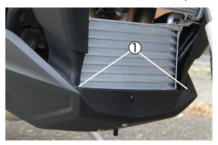
Use a small tool to push the centers out of the (2) OEM toggle fasteners. Make sure you recover the centers and keep them in a tray with the toggle heads.
