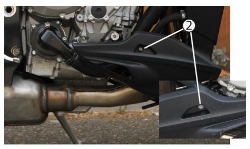
Use a t25 torx driver to remove the OEM fastener on the right side of the belly pan, then remove the fastener on the left side. Remove the pan and set it aside.
